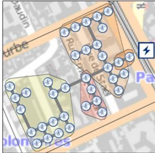
Figure 8 - Detailed MV network and aggregated clusters
