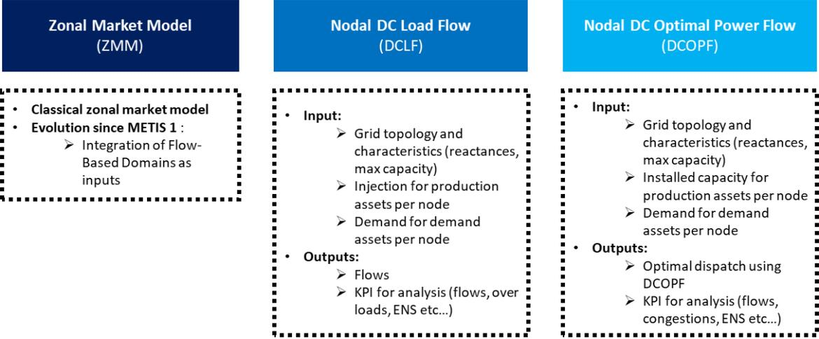
Figure 1 Three Main Models of the transmission module of METIS
