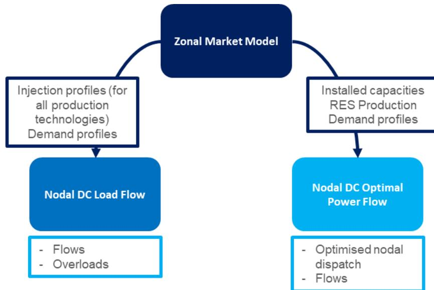
Figure 22 - Disaggregation from zonal to nodal model
