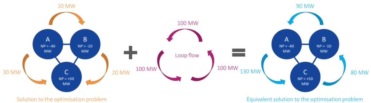
Figure 6 - Illustrative case of the equivalent solutions of one flow-based model without an additional constraint on the flows
