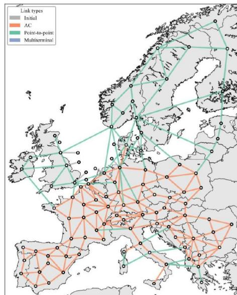
Figure 18 - Grid model and offshore production sites used in [8]
