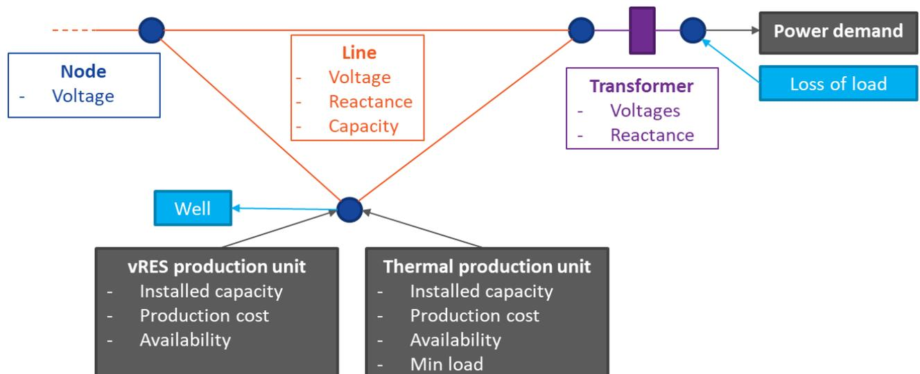
Figure 4 - Representation of a simplified transmission network
