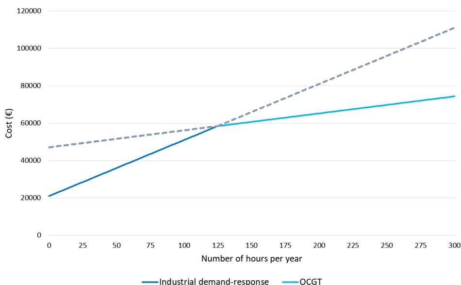
Figure 28 - Cost of industrial demand-response and OCGTs depending on the duration of use
