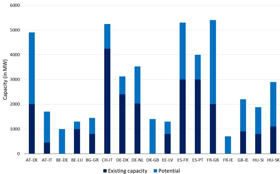
Figure 23 - Considered potential for additional interconnectors
