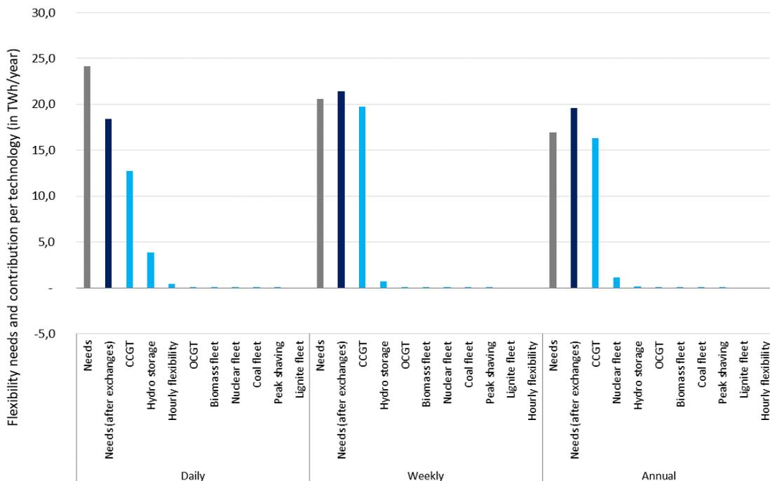
Figure 148: Contribution to flexibility needs per technology in Option (III)
