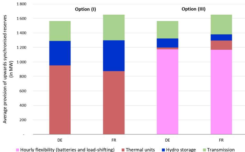
Figure 30 - Contribution of technologies to upwards synchronised reserve
