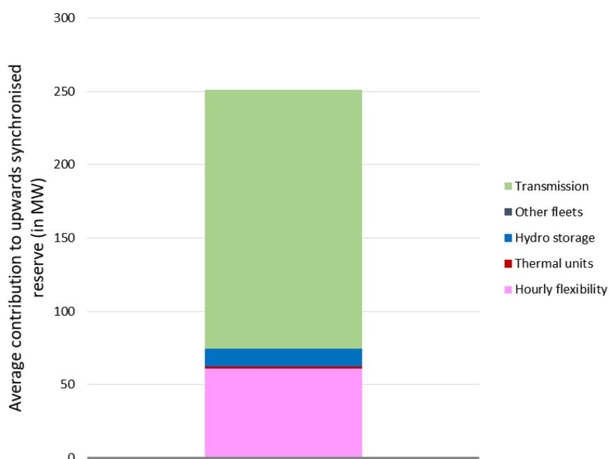
Figure 133: Contribution to upward synchronised reserve
