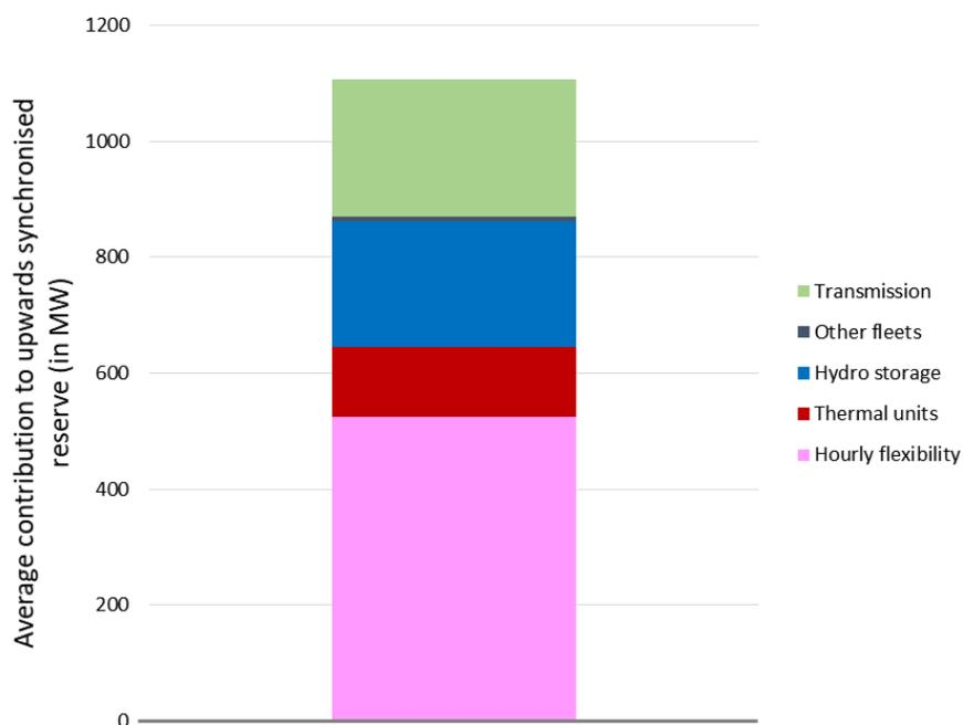
Figure 141: Contribution to upward synchronised reserve
