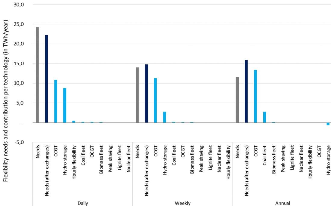
Figure 99: Contribution to flexibility needs per technology in Option (III)
