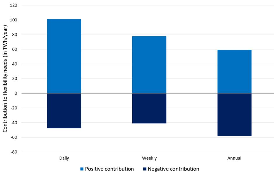
Figure 37 - Contribution of interconnectors to flexibility needs in EU28 in Option (III)
