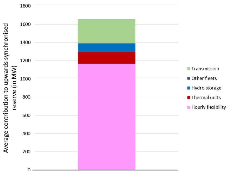
Figure 80: Contribution to upward synchronised reserve
