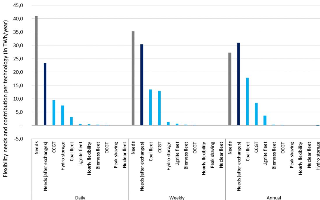
Figure 83: Contribution to flexibility needs per technology in Option (III)
