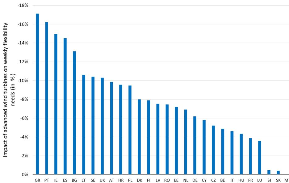
*Figure 35 - Mitigation of weekly flexibility needs due to the use of advanced wind turbines*
