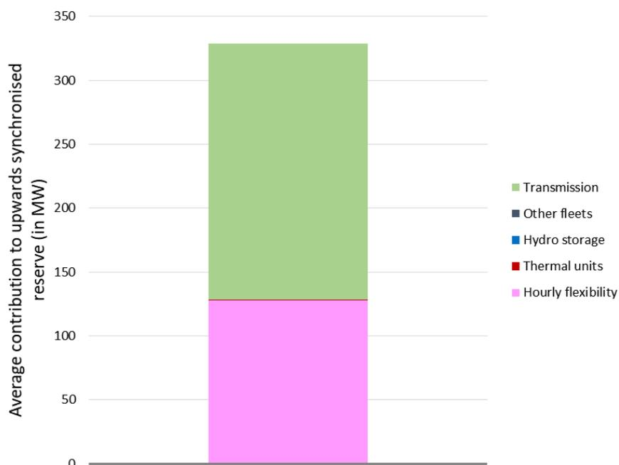
Figure 92: Contribution to upward synchronised reserve
