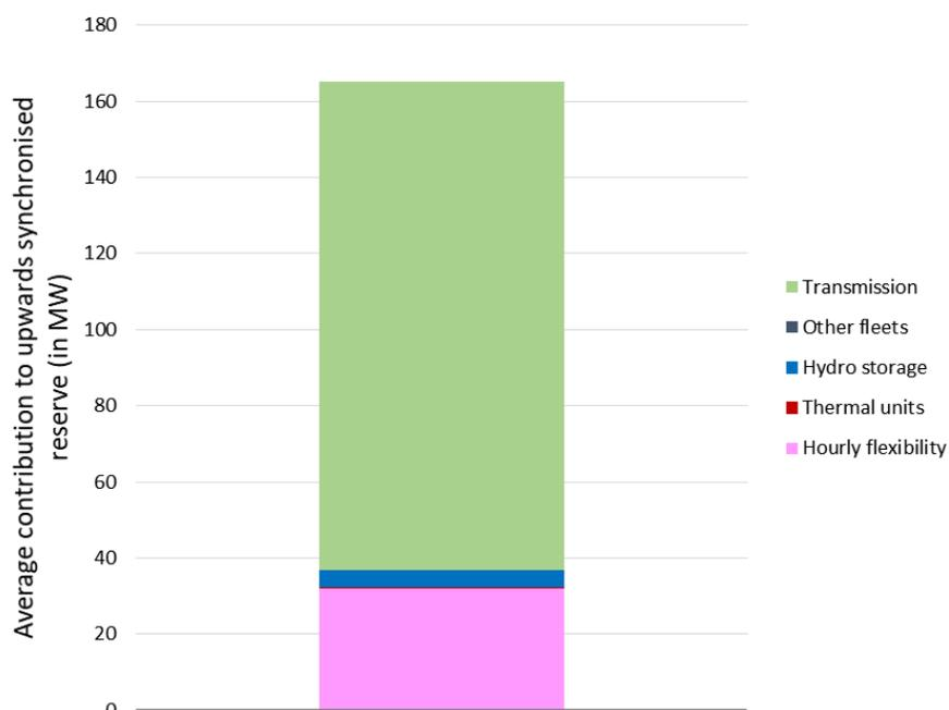
Figure 137: Contribution to upward synchronised reserve
