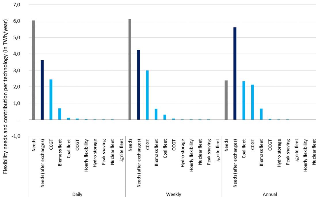
Figure 116: Contribution to flexibility needs per technology in Option (III)
