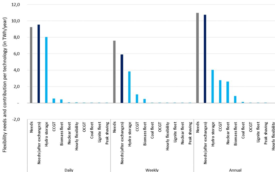
Figure 144: Contribution to flexibility needs per technology in Option (III)
