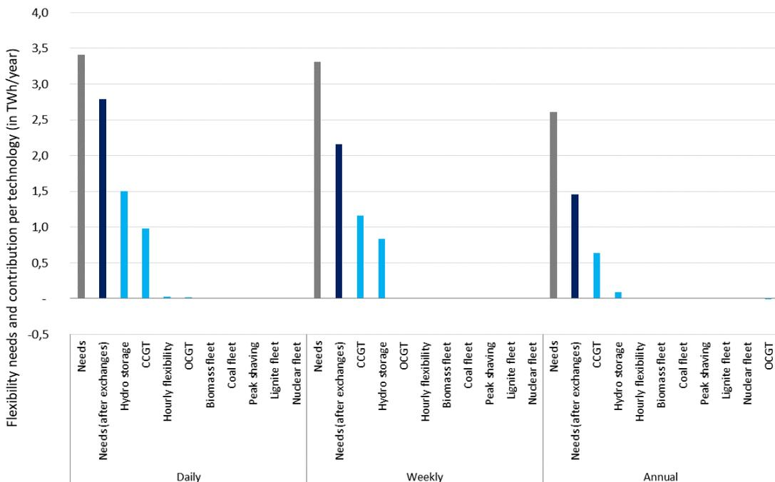
Figure 124: Contribution to flexibility needs per technology in Option (III)
