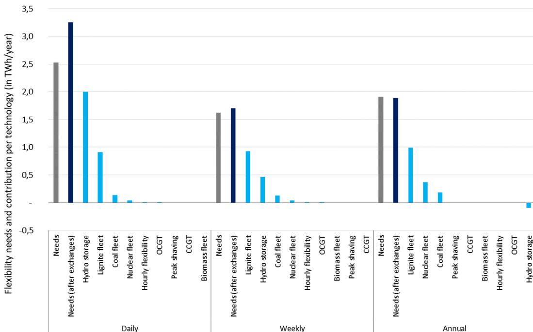
Figure 52 - Contribution to flexibility needs per technology in Option (III)
