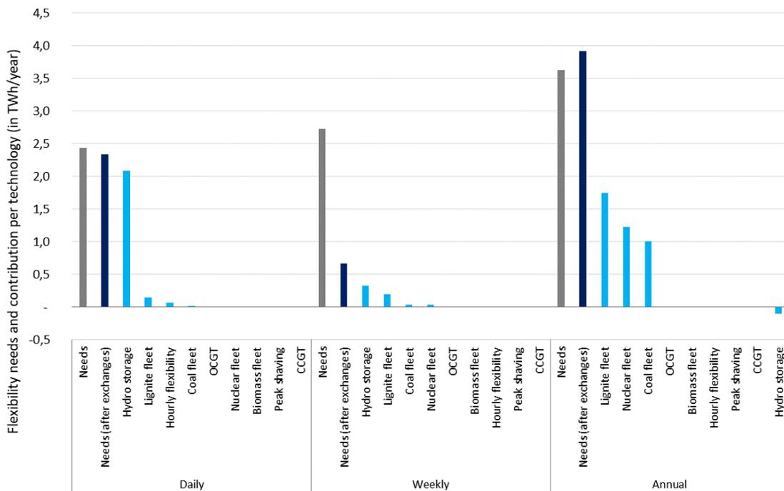
Figure 63: Contribution to flexibility needs per technology in Option (III)
