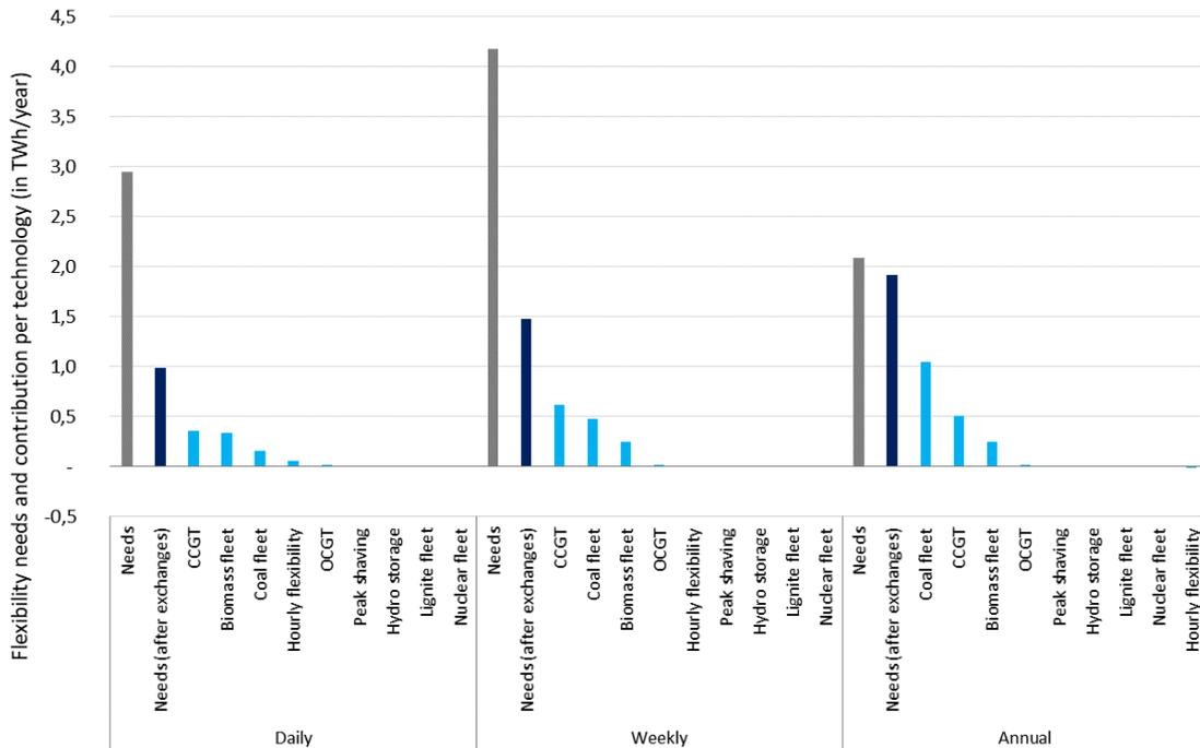
Figure 67: Contribution to flexibility needs per technology in Option (III)
