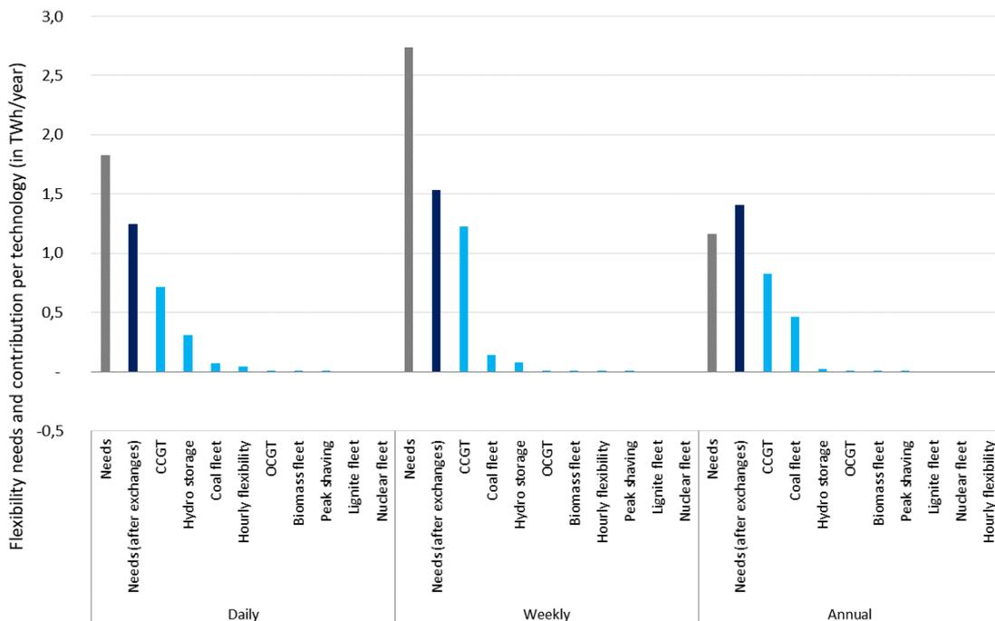
Figure 95: Contribution to flexibility needs per technology in Option (III)
