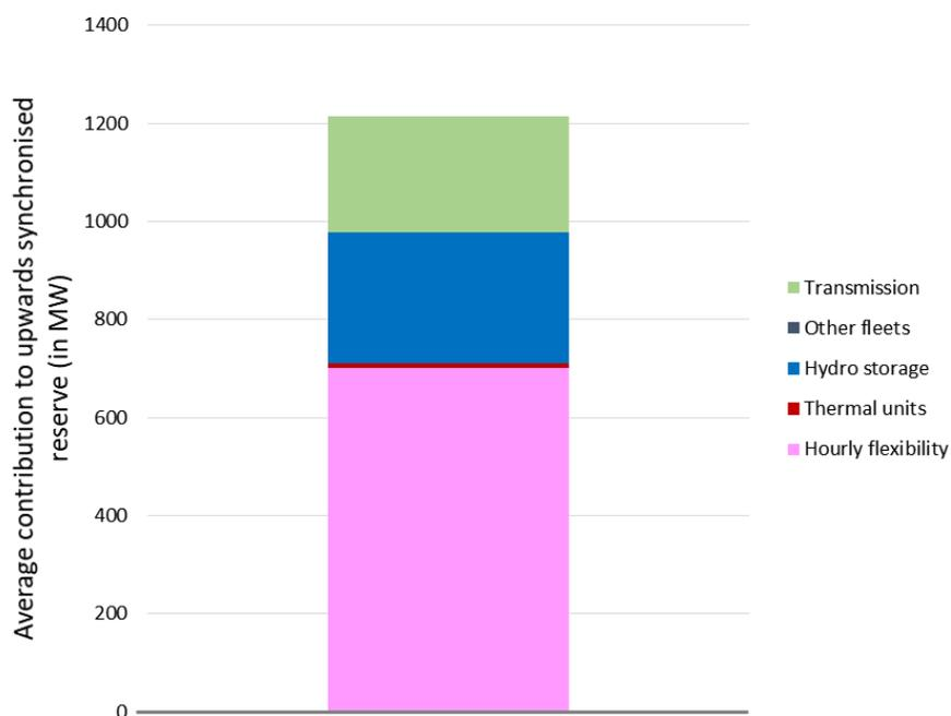
Figure 145: Contribution to upward synchronised reserve
