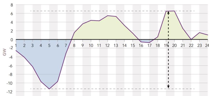
Figure 4 - Illustration of daily flexibility needs (the solid purple line measures the deviation of the residual load from its daily average for a given day). Source: RTE, Bilan prévisionnel de l'équilibre offre-demande, 2015
