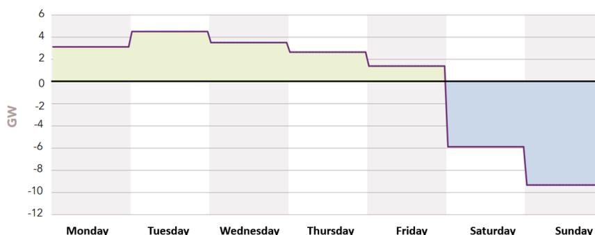
Figure 5 - Illustration of daily flexibility needs (the solid purple line measure the deviation of the residual load from its daily average for a given week). Source: RTE, Bilan prévisionnel de l'équilibre offre-demande, 2015
