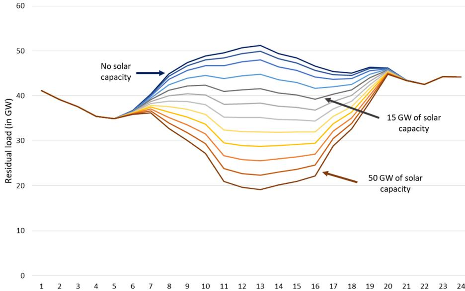
Figure 12 – Illustration of the impact of solar capacity deployment on the residual load
