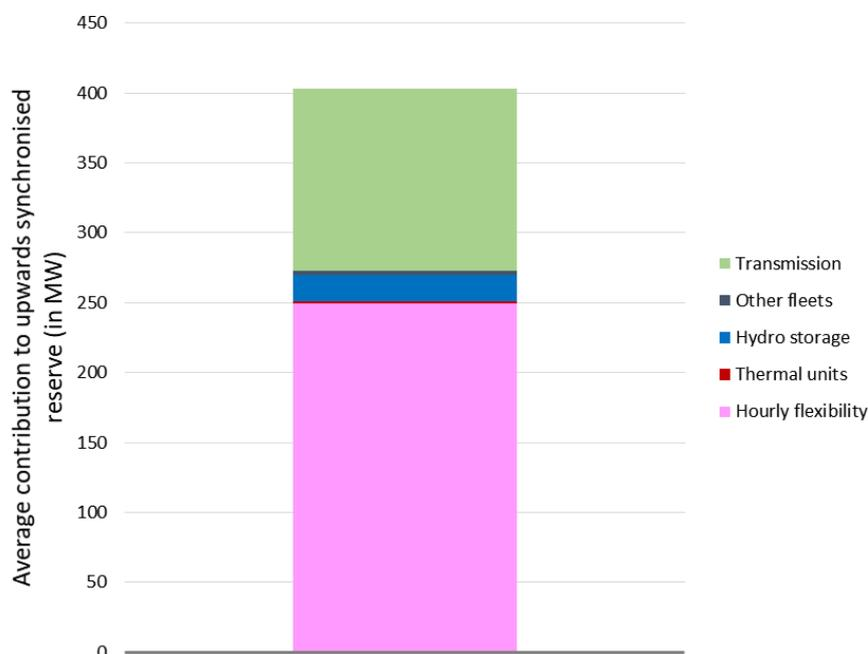
Figure 88: Contribution to upward synchronised reserve
