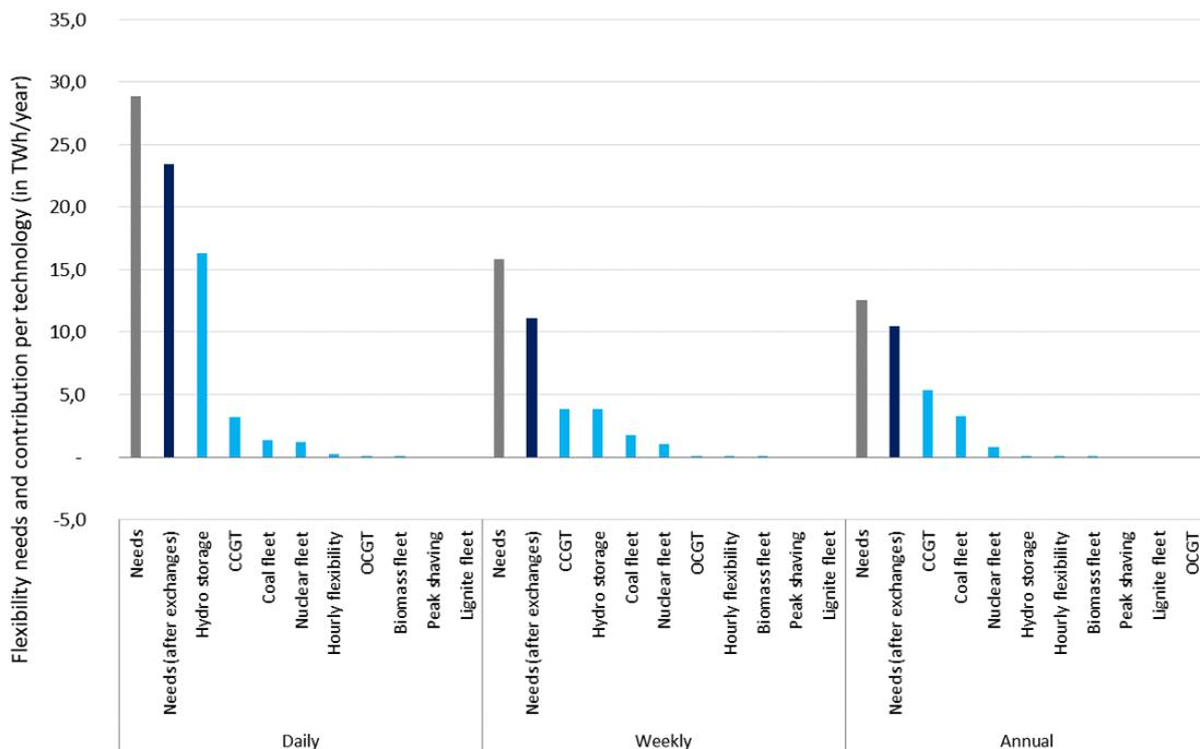
Figure 140: Contribution to flexibility needs per technology in Option (III)
