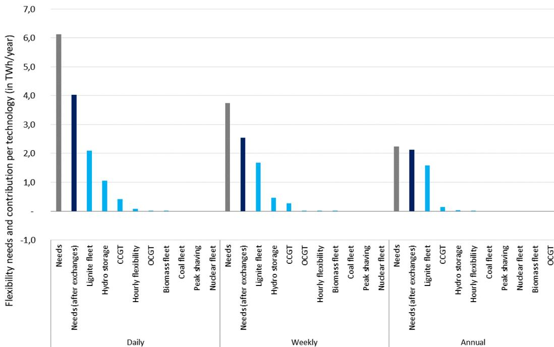
Figure 87: Contribution to flexibility needs per technology in Option (III)
