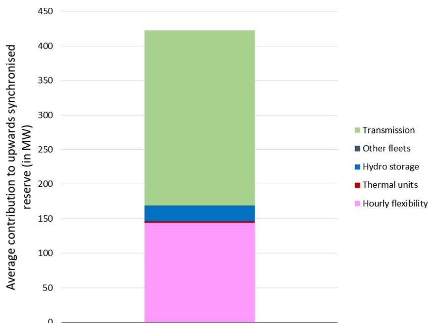
Figure 64: Contribution to upward synchronised reserve
