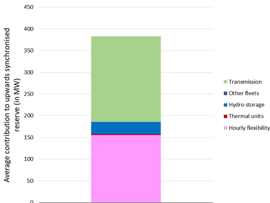
Figure 45 - Contribution to upward synchronised reserve
