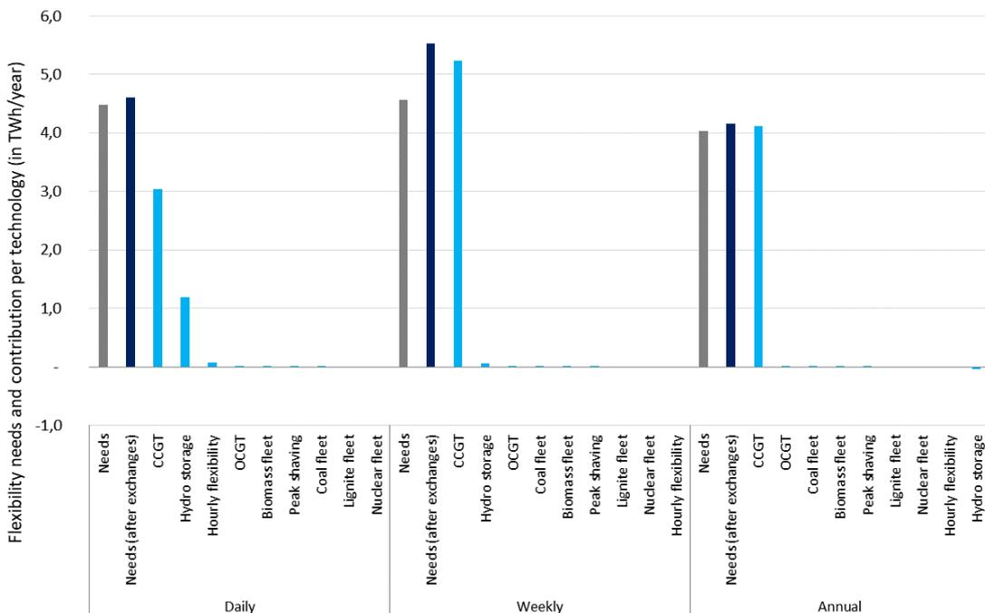
Figure 48: Contribution to flexibility needs per technology in Option (III)
