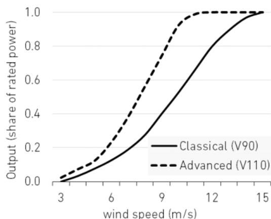
Figure 25 - Power generation according to wind speeds per turbine type. Source: Hirth, Lion & Simon Müller (2016): "System-friendly wind power: How advanced wind turbine design can increase the economic value of electricity generated through wind power", *Energy Economics* 56, 51-63
