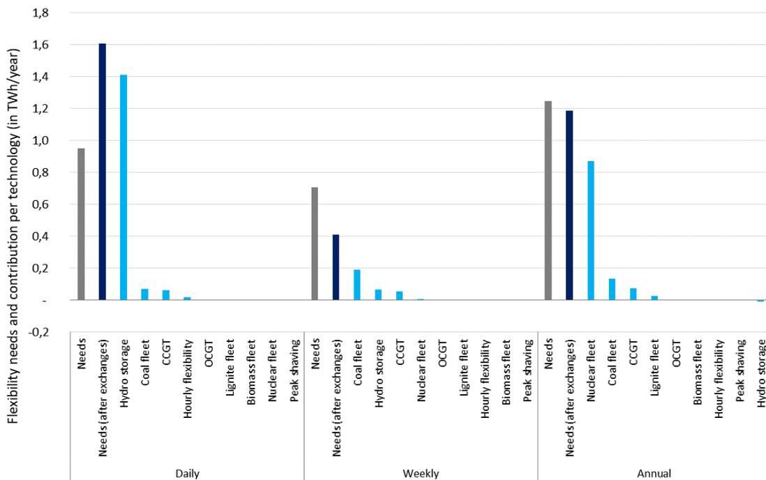
Figure 132: Contribution to flexibility needs per technology in Option (III)
