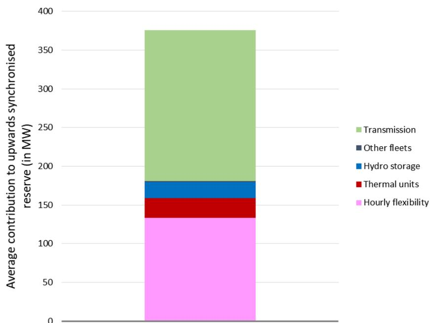
Figure 129: Contribution to upward synchronised reserve
