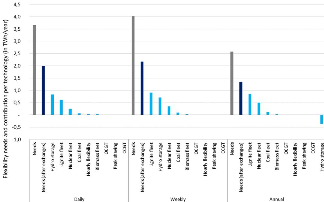
Figure 128: Contribution to flexibility needs per technology in Option (III)
