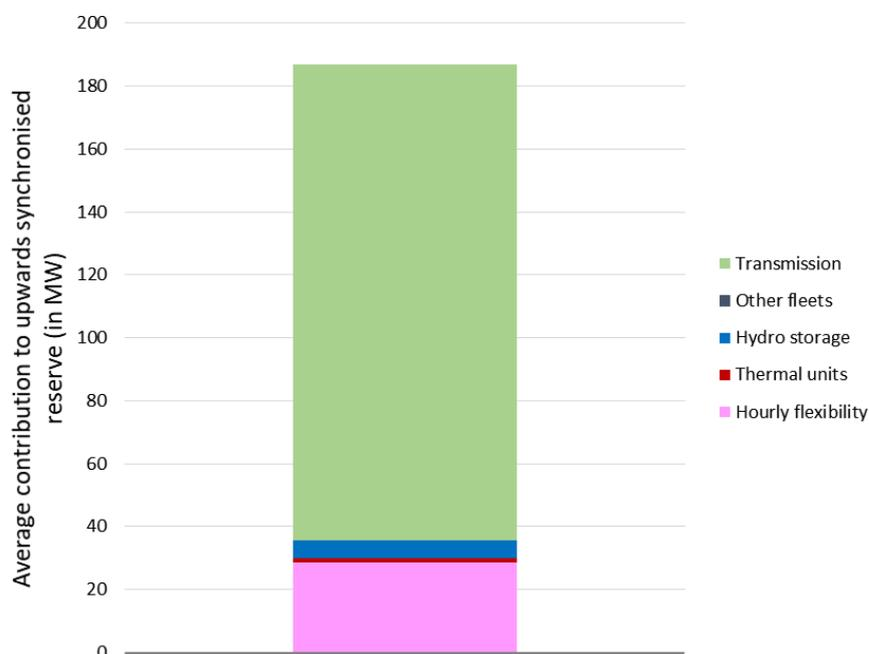
Figure 57: Contribution to upward synchronised reserve
