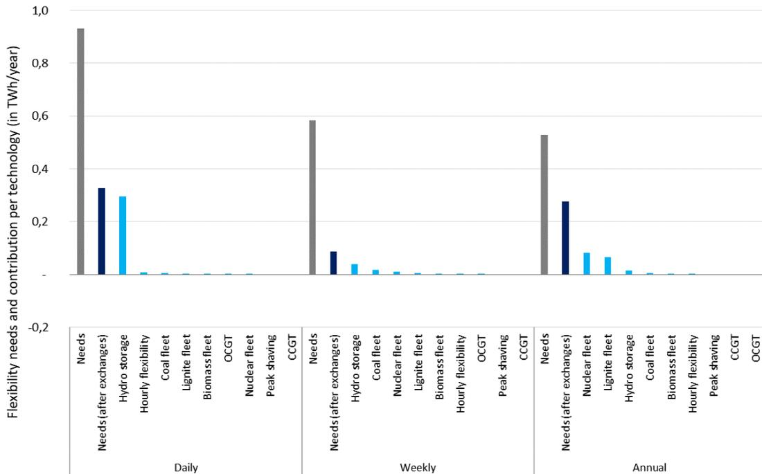
Figure 136: Contribution to flexibility needs per technology in Option (III)
