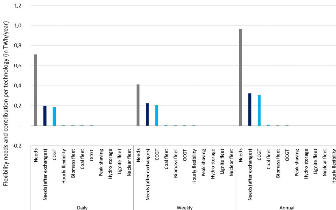
Figure 103: Contribution to flexibility needs per technology in Option (III)
