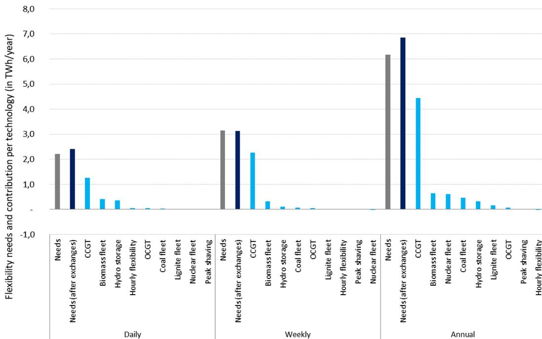
Figure 75: Contribution to flexibility needs per technology in Option (III)
