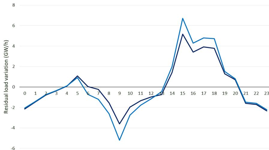
Figure 6 – Illustration of the residual load variation in two scenarios with different RES-e shares. The light blue scenario (high RES share) requires more ramping than the dark blue scenario (low RES share)
