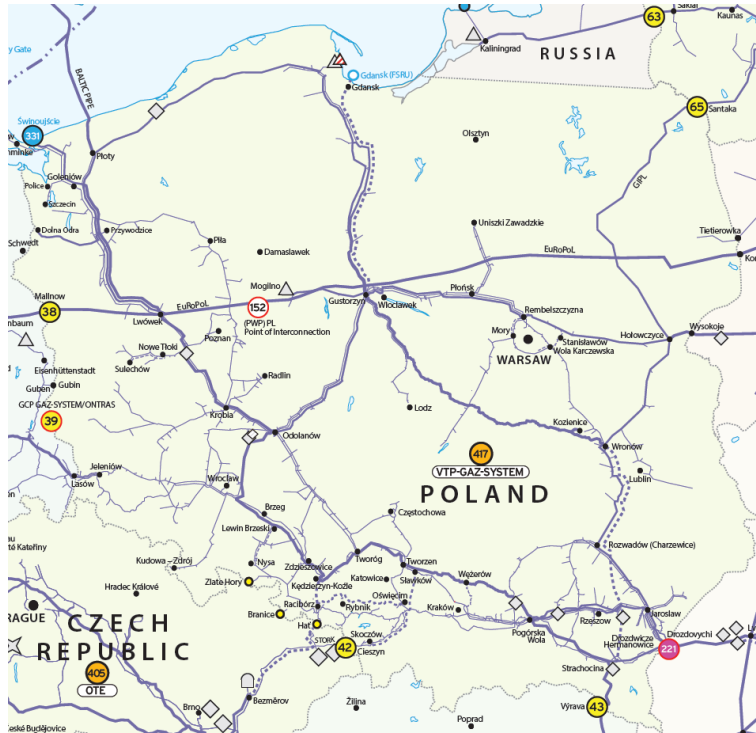
Figure 9-2 Current and planned gas infrastructures in Poland (Source: ENTSOG)
