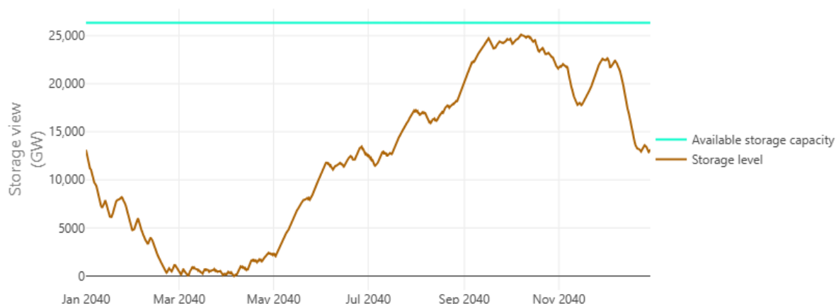
Figure 5-22 Hydrogen storage levels in 2040 in the baseline scenario
