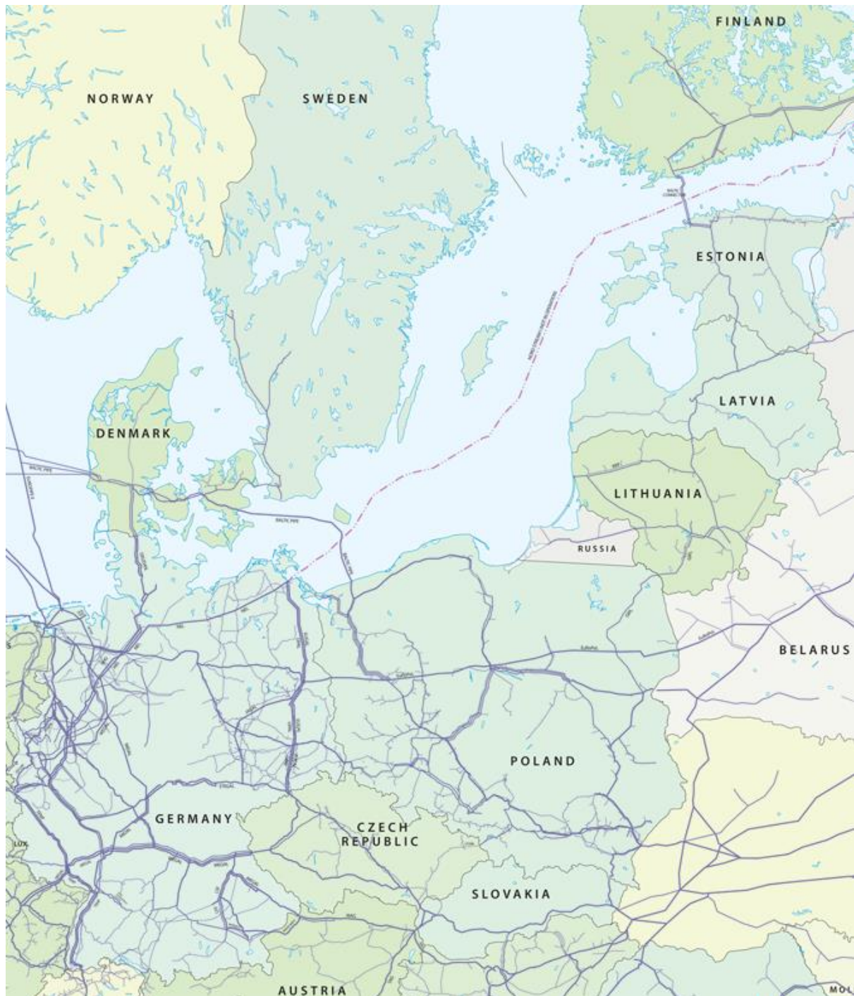
Figure 3-1 Gas transmission infrastructure in the BEMIP region (Source: ENTSOG Transparency Platform) 49
