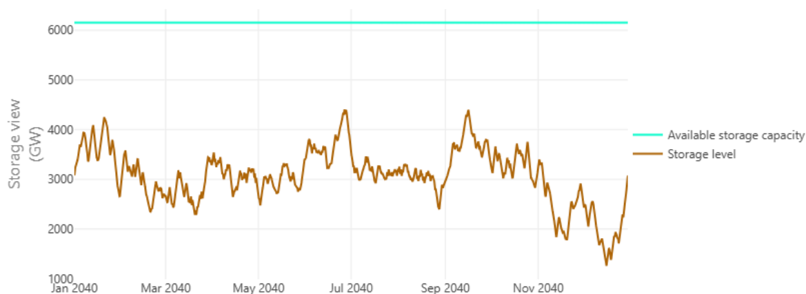
Figure 5-23 Hydrogen storage levels in 2040 in the sensitivity scenario
