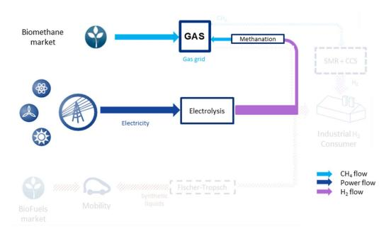
Figure 24 - Schematic overview of use case 2: power-to-CH<sub>4</sub> vs biomass-to-CH<sub>4</sub>
