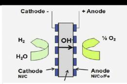
Figure 9 - Illustration of the operating principle of an alkaline water electrolysis cell [31]
