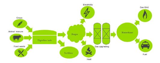
Figure 14 - Schematic overview of the anaerobic digestion process [19]
