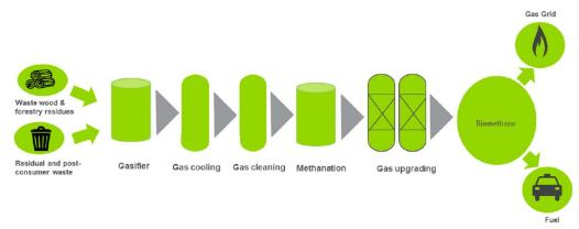
Figure 15 - Schematic overview of the thermal gasification process [19]
