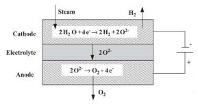
Figure 11 - Illustration of the operating principle of SOEC [32]
