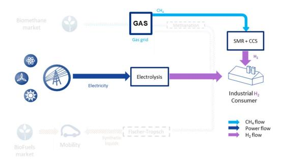
Figure 22 - Schematic overview of use case 1: power-to-H<sub>2</sub> vs SMR + CCS
