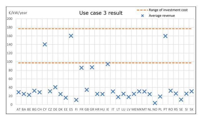
Figure 34 - Average annual compared to the annual investment cost for power-to-Liquids in the case of competition with biomass-to-Liquids (production cost of biofuel =  $75 \text{ €/MWh}_{PLL\ HHV}$ )
