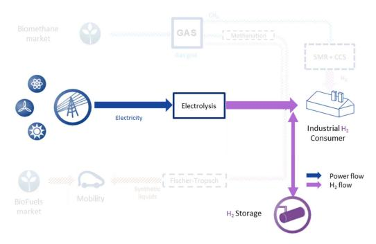
Figure 23 - Schematic overview of variant use case 1: power-to-H<sub>2</sub> + H<sub>2</sub> storage
