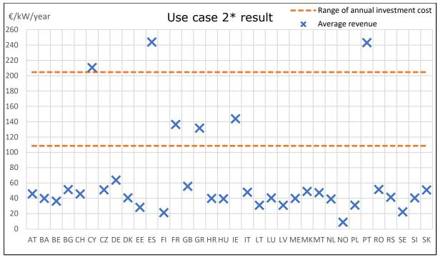
Figure 33 - Average annual revenue compared to the annual investment cost for power-to- $CH_4$  in the case of competition with biomass-to- $CH_4$  (production cost of biomethane = 106  $\bigcirc$ /MWh<sub>CH4</sub> HHV)
