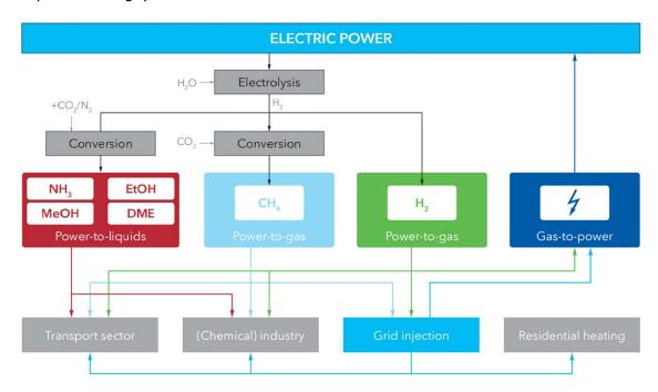
Figure 1 - Schematic representation of power-to-X [1]
