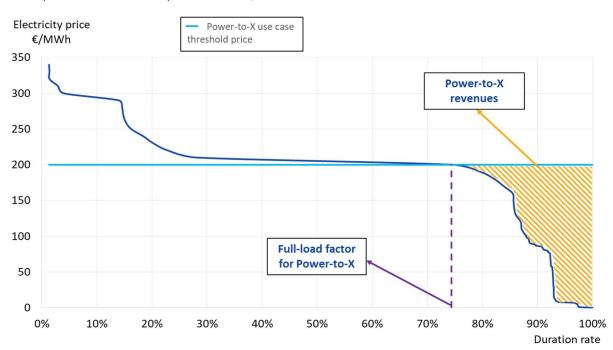
Figure 21 – Power-to-X full-load factor versus the threshold electricity price to use power-to-X. Example with a threshold price of 200 €/MWh.
