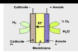
principle of a PEM water electrolysis cell [31]
